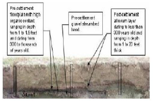
Trench excavated across the existing floodplain reveals the presettlement streambed and floodplain levels currently buried under post-settlement alluvium and facilitates soil layer analyses, including various dating procedures.
